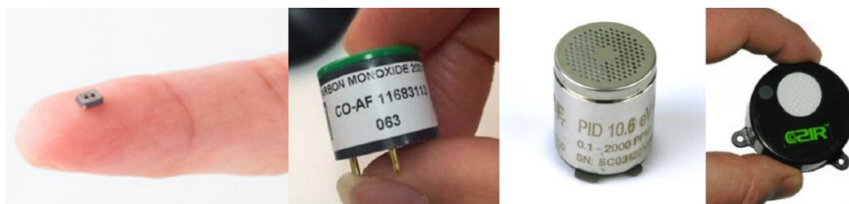
Figure 4. Examples of low-cost chemical sensors. (from left to right) MOX sensor (Model: FigaroTGS 8100); AGS sensor (Model: Alphasense CO-AF); PID (Model: RAE Systems PID 10.6 eV); (d) NDIR sensor (Model: CozIR by Gas Sensing Solutions) [50].
